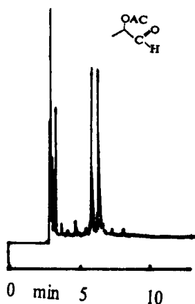
Fig. 3. Enantiomer separation of 2-O-acetylated propion aldehyde. Column temperature 150°C.
